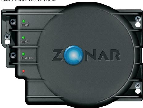
Zonar's HD-GPS main chipset maintains a very high sample rate, 1 sample per second or higher. The hardware is designed to detect vehicle position and velocity using a 12 channel GPS receiver and then re-compute distance traveled at every sample. The device logs latitude, longitude, time, event and odometer at every log data point.
